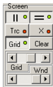
Fig. 4.3.1. – The cursors and grid controls
