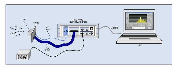
In a typical setup the Hamamatsu H8711 PMT is plugged into the SIB116 Sensor Interface Board which in turn connects to a Vertilon PhotoniQ IQSP480 or IQSP580 multichannel data acquisition system using a SIB cable. When triggered from an external source, the PhotoniQ integrates and digitizes the 16 charge signals from the H8711 and outputs a data packet to the PC over a USB connection. The PhotoniQ also supplies the PMT high voltage bias through a specialized high voltage cable.
