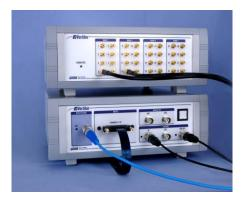
The photo shows an SDS232 connected to a PhotoniQ IQSP480 32-channel PMT / APD data acquisition system. Two channels of the SDS232 are connected to single element silicon photomultiplier (SPM) devices.
