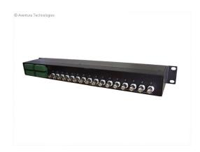
• 16 Port Passive Transceiver Hub In 1U Rack Mountable Panel
