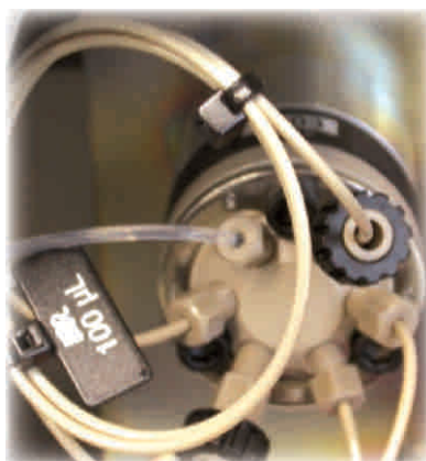
Exchangeable Sample Loop made of PEEK
